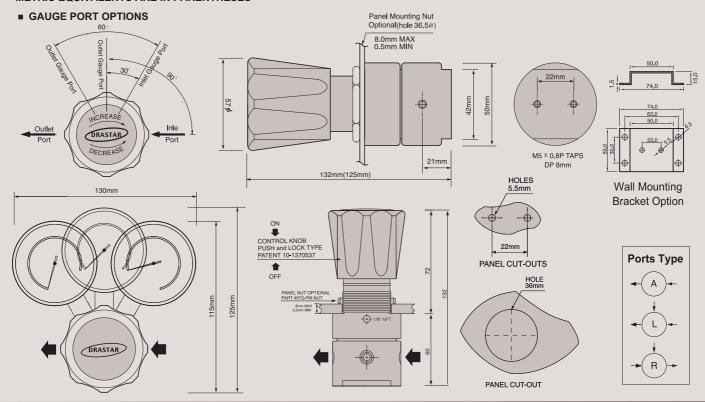
077 Series is a 1/4" NPT type relief/back-pressure regulator suitable for water, chemical, liquid, gas, etc. Regulator's body is made of brass or stainless steel 316L (077S) and 077 Series can be used for very low pressure of 0.3bar (5psig) up to 20 bar (290 psig).
